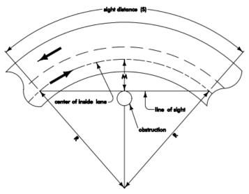
curve is 365 feet. This distance is based on a minimum of 4 feet clear of obstructions beyond the road.
